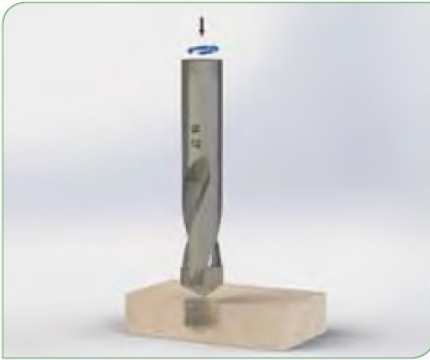
1 Prepare the hole in the receiving material.
