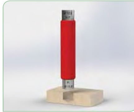
2 Check the correct hole dimension with a go/no go gauge.
