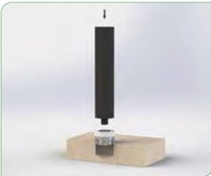
3 Install the insert by pressure.
